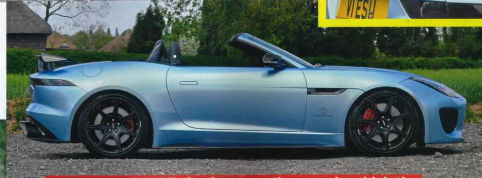
BELOW: With the suspension lowered by 20mm, the big Dymag carbon fibre wheels fill the arches
